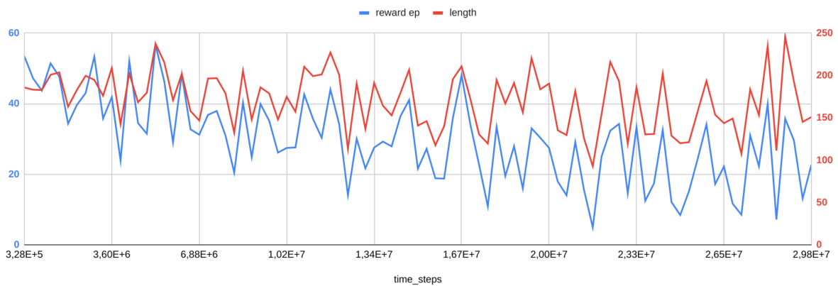
Figura 5.5: Training the Dribble skill with the regular reward (4.3). Graph of the Reward (blue) and Length (red) of an episode of training as the time-steps increases (x-axis)
